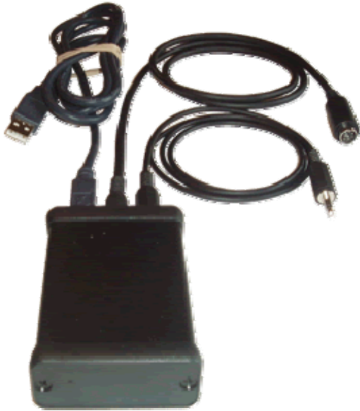
DigiMaster Dual Channel USB MultiFace, Shown above with 1 Icom CAT/CI-V lead and 1 Yaesu Y3 CAT cable for the FT857.
